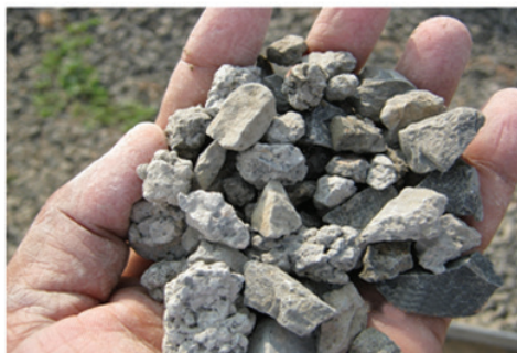
Fig. 1: Unprocessed Recycled Aggregate
